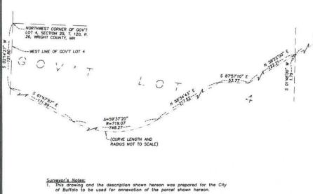
2. No field work was performed for the preparation of this drawing and description. The following sources were utilized: Plats and documents of record, information in our files from previous surveys, section breakdown
